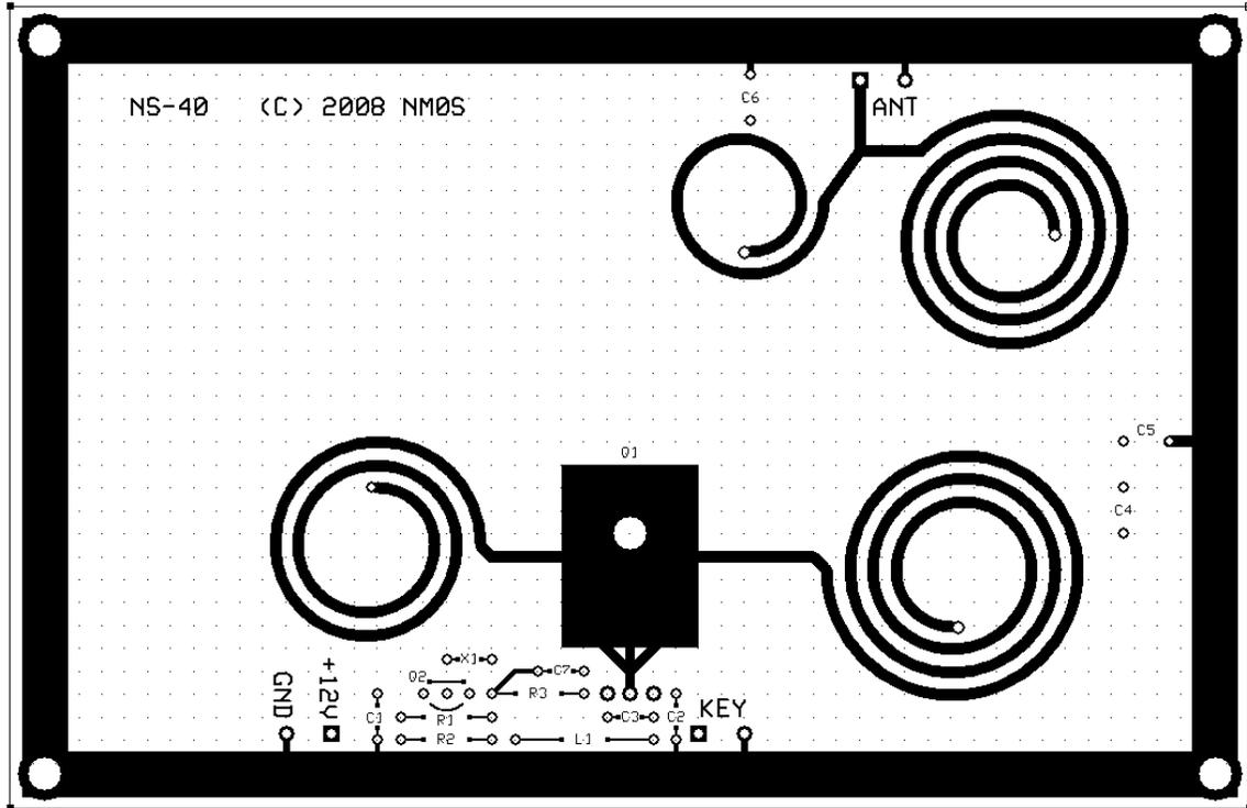
Figure 2: Component Placement on the PC Board
