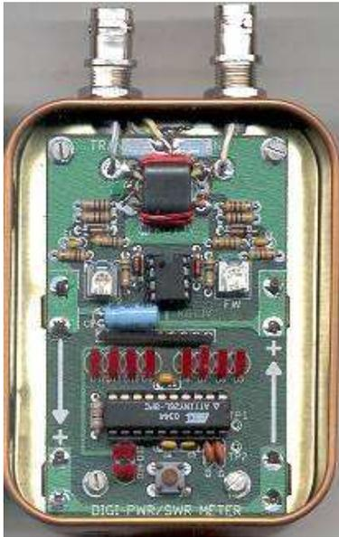
If packaging in a Whitman's tin, you will want to mount the LED's flush to the board. Also, the electrolytic, C8, will need to be mounted lying on it's side. Mount the board with threaded spacers, so that you may more easily gain access to the batteries under the board. 1/2" spacers are a tad (1/16") too short, so use a lock washer or nut for additional spacing. 4/40 spacers will short circuit to
