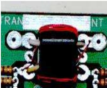
A short piece of #22 Teflon insulated stranded wire is passed through the hole of the core, then soldered to the adjacent pads. This secures the core to the board and forms the primary winding.
